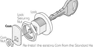
Re-Install the existing Cam from the Standard Key Lock to the "Random" Key Lock
